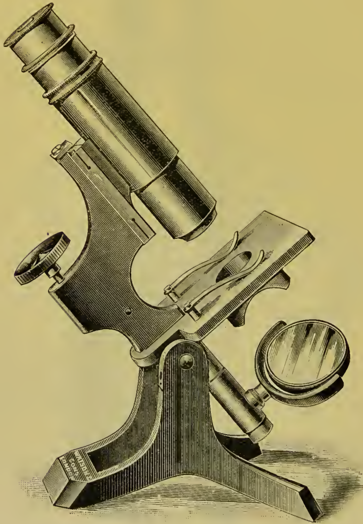
Fig. 74.—Watson's Histological Microscope. Stand "A."—Height, when placed vertically and tube pushed home, 9\frac{1}{2} inches.
